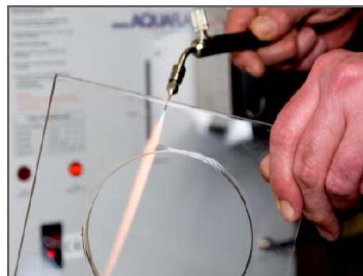
Flame polishing of acrylic edge
